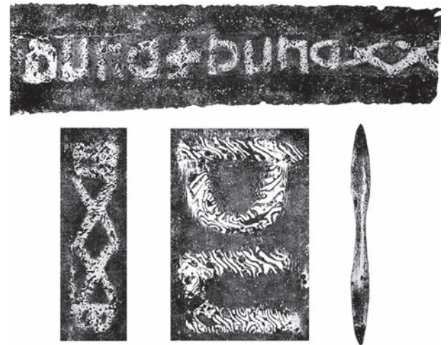
Fig. 6. Types of patterns distinctive to pattern-welded swords. Drawing by P. Kucypera.
